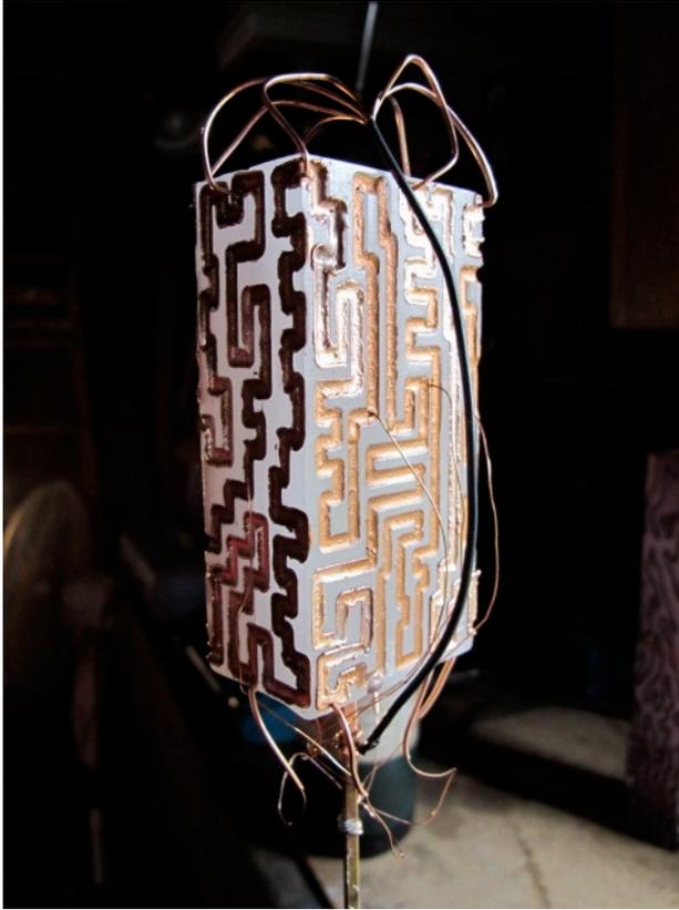
Figure 37. Wax mandrel for *Labyrinth 110501* showing milled channel painted with conductive coating. Electrodes connect channels to circuit of electroforming
